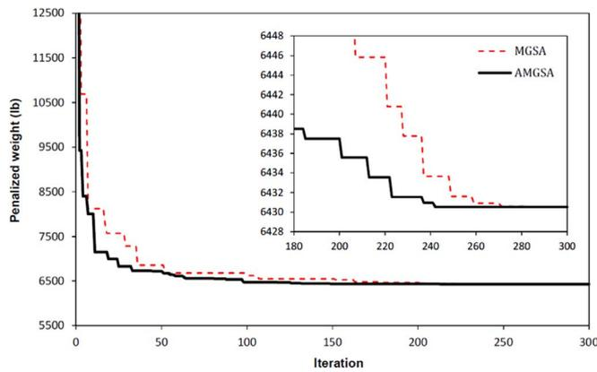
Fig. 6. Convergence histories of MGSA and AMGSA for the 18-bar truss.
