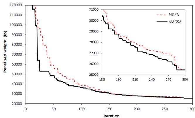
**Fig. 10.** Convergence histories of MGSA and AMGSA for the 200-bar truss.
