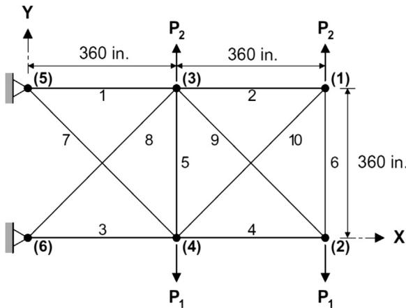
Fig. 3. The 10-bar planar truss.
