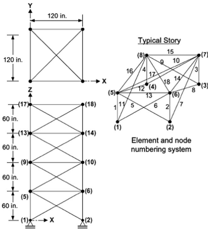
Fig. 7. The 72-bar space truss.
