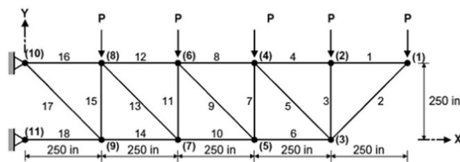
Fig. 5. The 18-bar planar truss.
