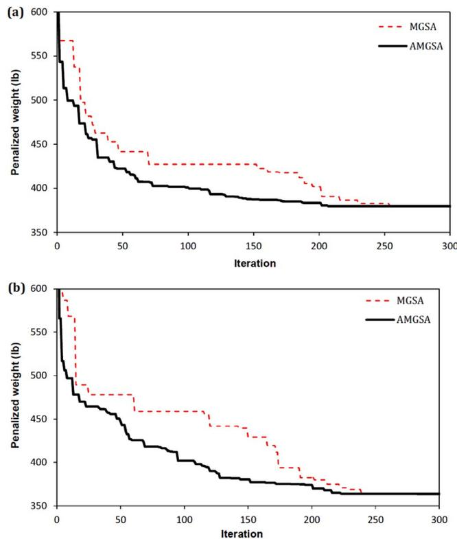
Fig. 8. Convergence histories of MGSA and AMGSA for the 72-bar truss under a) Case 1 and b) Case 2.
