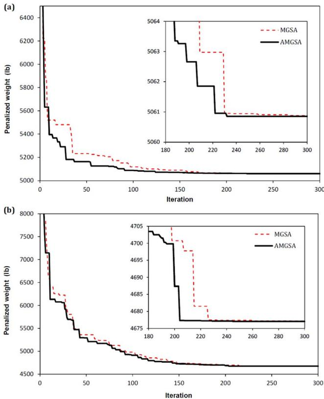
**Fig. 4.** Convergence histories of MGSA and AMGSA for the 10-bar truss under a) Case 1 and b) Case 2.
