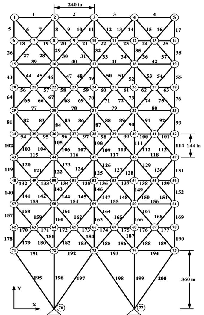
Fig. 9. The 200-bar planar truss.
